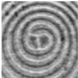
Rolls and hexagons in thermal convection
