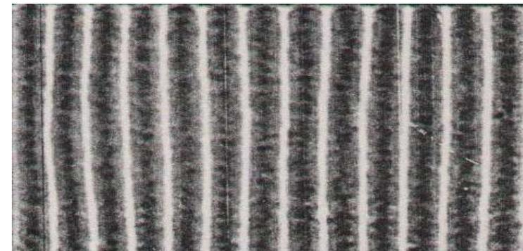
Visualization by illuminating from below (index of refraction changes with temperature periodically).
