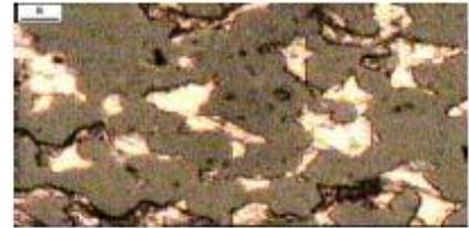
Microstructure of the boron carbide (dark)-Copper (bright) composite.
